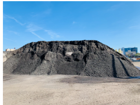
(b) Recycled Asphalt Pile
