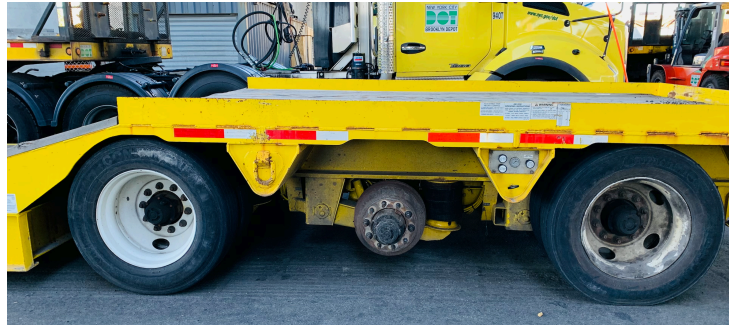
Figure 16 – Imbalance Weights of the Tandem Axle (Truck R2, Class 9 3S2 Split)
